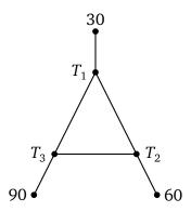
Let  $T_1$ ,  $T_2$ ,  $T_3$  be the temperatures at the interior points. Assume the temperature at each interior point is the average of the temperatures of the three adjacent points.
